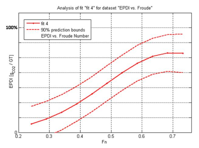
EPDI: Installed power divided by the gross tonnage and plotted against the Froude number.
